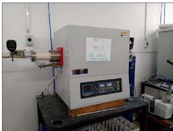
Figura 4. Horno tubular Thermoelectric Inc TH1200.
